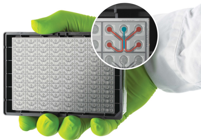
FIGURE 1. Schematic presentation of the MIMETAS OrganoPlate® 3-lane 64
